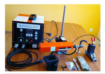
Order No.: EDM RBT1 EDM device for removing broken taps
