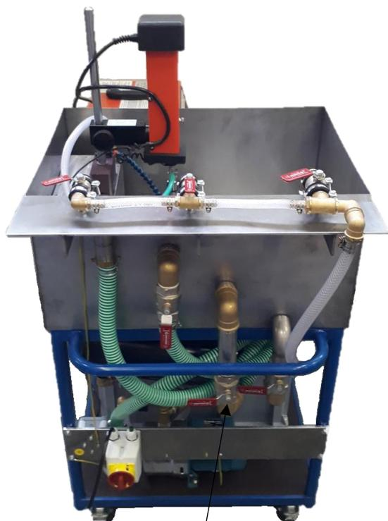
Set of valves and overflow for pouring working liquid out from work tank, in 4 different levels: 0mm, 100mm, 200mm, 305mm
